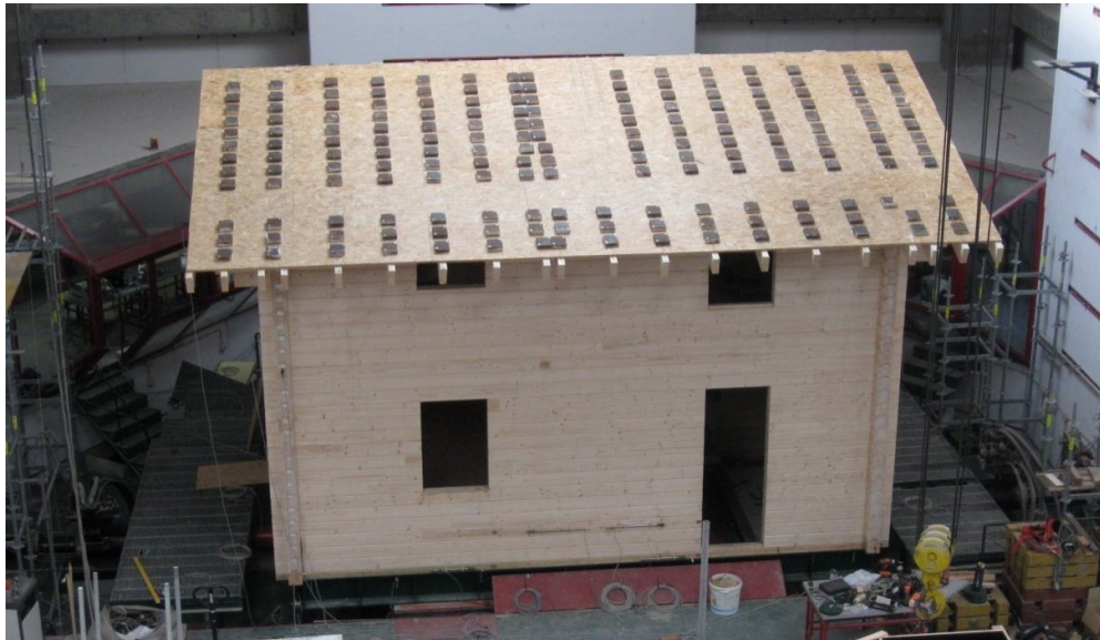
Figure 3 —The fully assembled house on the shaking table
