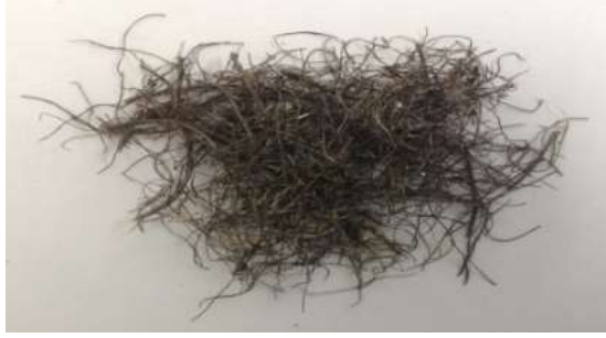
Figure 2. Recycled steel fibres extracted from wasted tires
