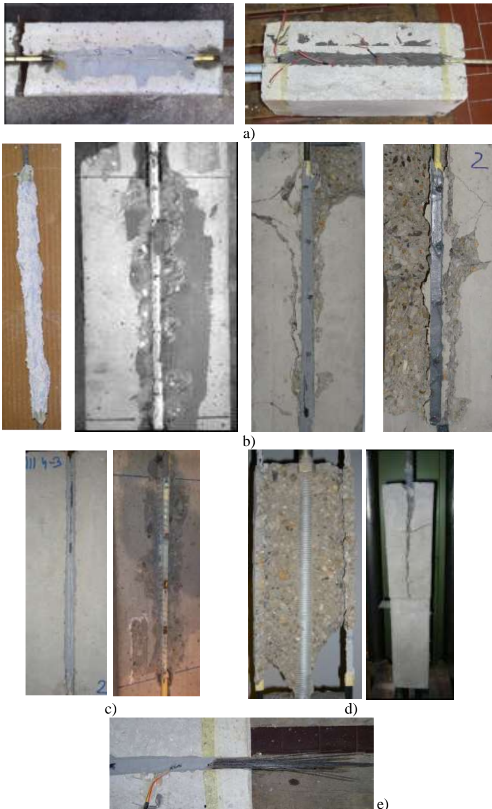
651 Figure 5. Examples of experimentally observed failure aspects: a) Debonding at the FRP- 652 adhesive interface (DB-FRP/A); b) Debonding at the concrete-adhesive interface, with various 653 degrees of concrete damage (DB-C/A); c) Adhesive splitting failure (SP-A); d) Splitting failure 654 of the concrete along the plane of the internal steel bars (SP-C); e) Tensile failure of the FRP (T- 655 FRP).
