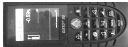
Fig. 2 - Reading gradient value with DISTO D83
