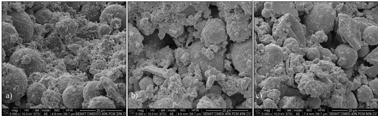
Fig. 4: Microstructure of cement mortars with incorporation of PCM and fly ash: a) 20% of fly ash (C400FA100-40PCM-F), b) 40% of fly ash (C300FA200-40PCM-F), c) 60% of fly ash (C200FA300-40PCM-F).
