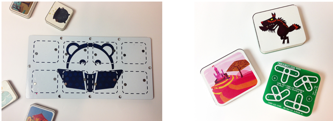
Fig. 3.3. Electronic platform with Bluetooth (left), back and front side of blocks (right).
