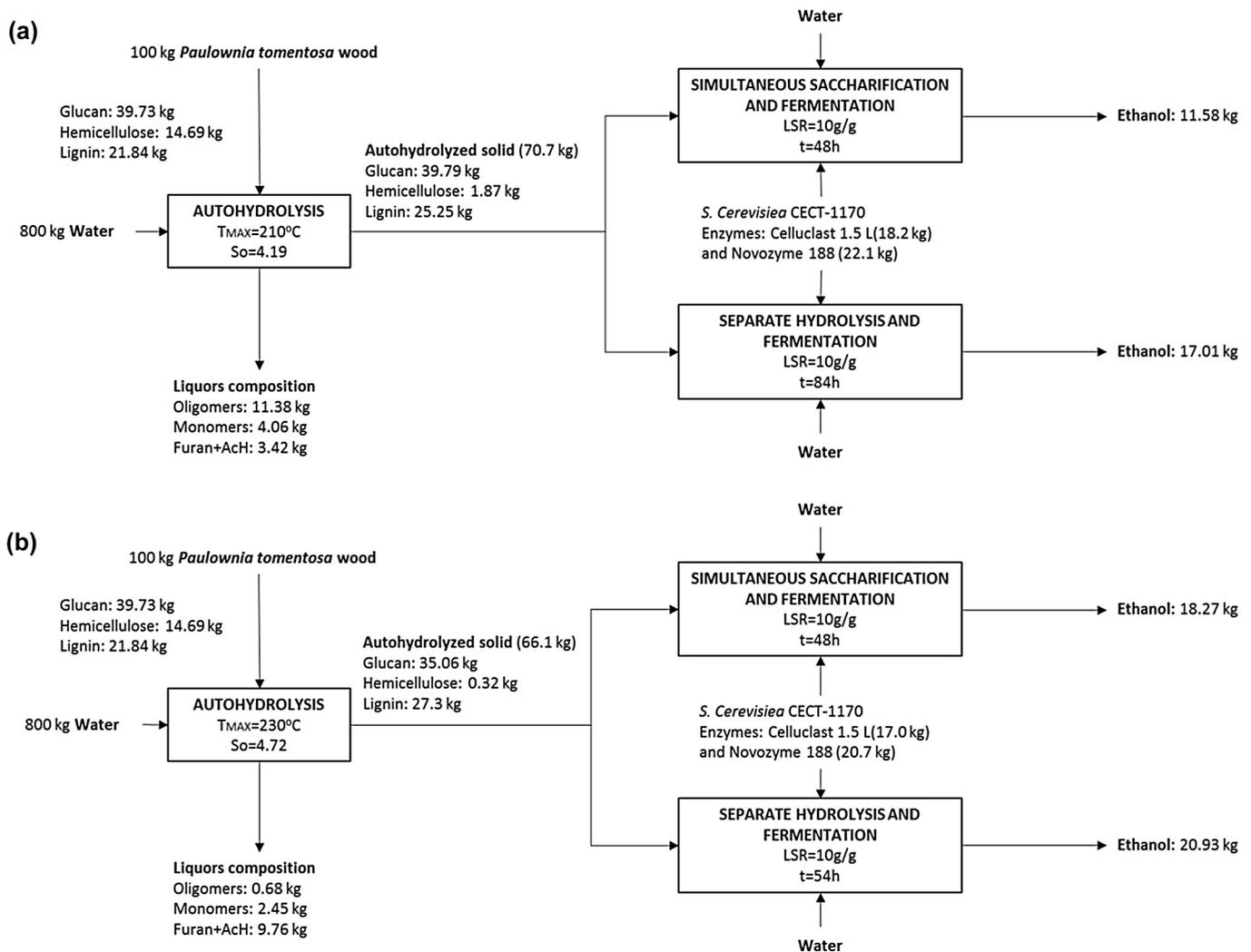
Fig. 7. Overall balance of Paulownia wood processing by autohydrolysis and saccharification and fermentation simultaneously and separately at severity conditions of pretreatment: (a)  $S_0 = 4.19$  and (b)  $S_0 = 4.72$  (results expressed in kg/100 kg raw material, oven dry basis).
