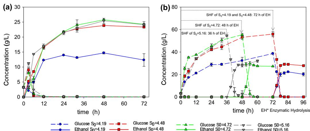
**Fig. 5.** Ethanol and glucose concentration (g/L) obtained from Paulownia (treated at  $S_0$ :4.19–5.16) by: (a) SSF process and (b) SHF process. Experiments were carried out in duplicate, error bars represented standard deviation.
