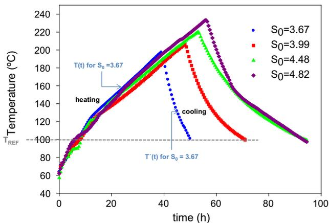
Fig. 2. Heating and cooling temperature profiles of autohydrolysis assay carried out at  $S_0 = 3.67, 3.99, 4.48$  and  $4.82$ . Temperature was controlled with a thermocouple inserted in a thermowell, which extends near the bottom of the reactor vessel ( $T(t)$ : heating profile,  $T'(t)$ : cooling profile,  $T_{REF}$ : temperature of reference,  $100\text{ }^\circ\text{C}$ ).
