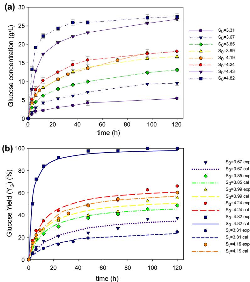
Fig. 3. (a) Time course of glucose concentration (g/L) of *Paulownia* wood treated at autohydrolysis conditions of  $S_0$  in the range: 3.31–4.82; (b) Yield of glucose (%) at autohydrolysis conditions of  $S_0$  in the range: 3.31–4.82. Experiments were carried out in duplicate, error bars represented standard deviation.
