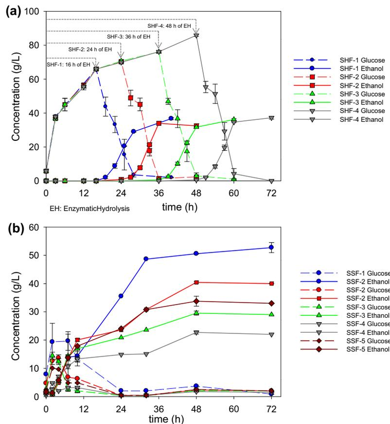
**Fig. 6.** a) Time course of ethanol concentration (g/L) from Paulownia wood treated at  $S_0 = 4.72$  (a) by SHF process varying the time of enzymatic hydrolysis step and (b) by SSF process. Experiments were carried out in duplicate, error bars represented standard deviation.
