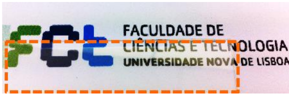
Fig. 5- Glass substrate with a transparent ZnO thin film deposited by RFMS
