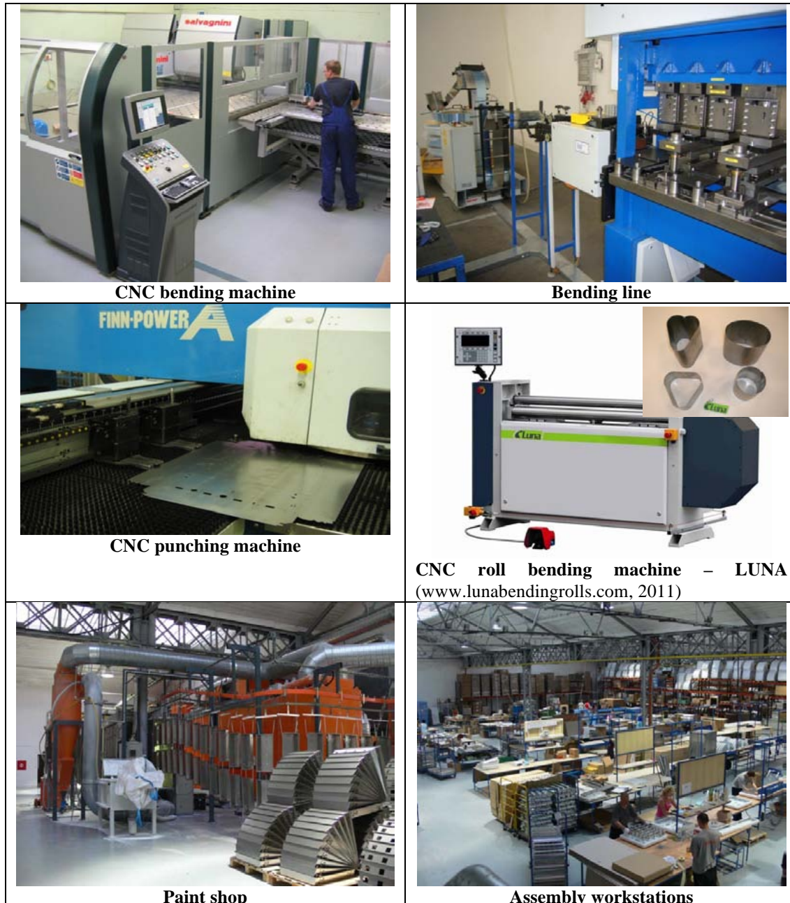
Figure 4 - Images from metal-forming and production areas
