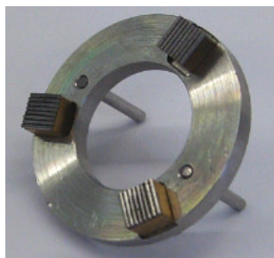
Fig.3 - Upper body with three contact surfaces
