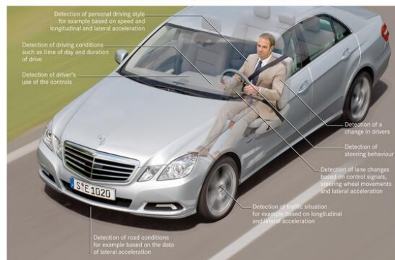
Attention Assist: How the Mercedes driver assistance system detects tiredness
