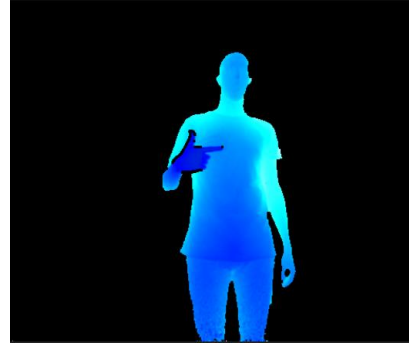
Figure 21 – Kinect sensor depth input after application of the background subtraction process. With background subtraction - the body silhouette becomes the only visible object, as it is the only object that moves in the Kinect sensor field of view.
