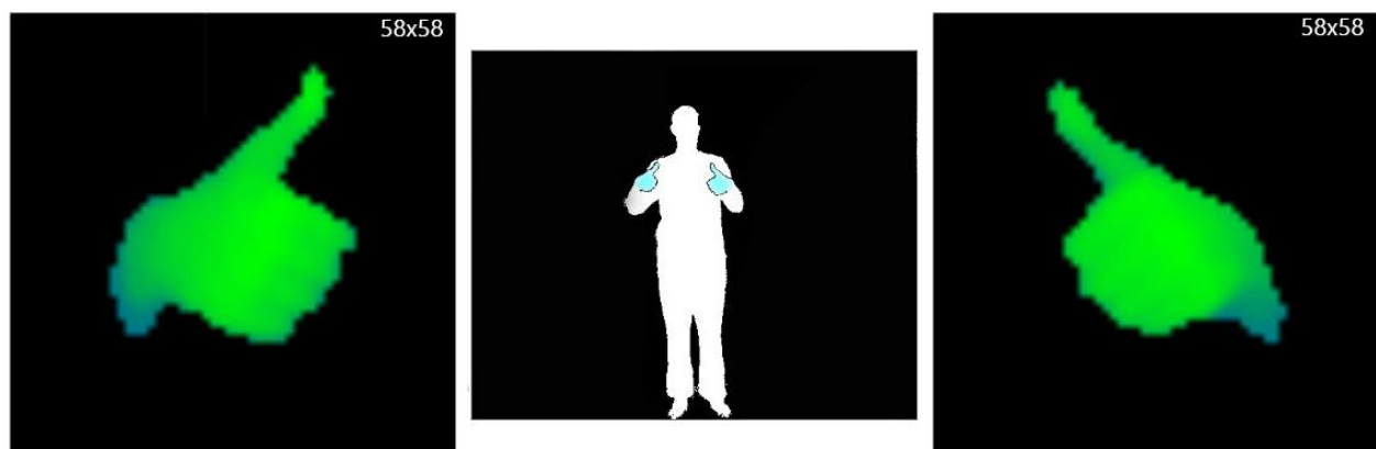
Figure 30 – Depth data input for the both hands. At the left side is the left hand and at the right side the right hand. The middle image is the original depth input after applying the background extraction. At the top right corners we depict the original size of the hand image. The colour representation is merely visual since the input for depth values varies from 0 (the sensor) to the max range the sensor can infer depth (accurately this range goes up to 4.5 m, hence 4500).
