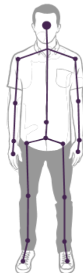
Figure 16 – Example of a standing pose (Microsoft, 2014b) to initiate data collection. The back and legs stay straight, both arms fall along the torso
