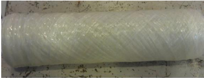
Figure 7. A successfully filament wound pipe produced by using the new developed equipment.
