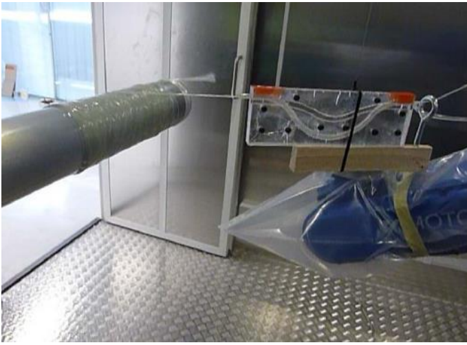
Figure 2. Syphon impregnation unit applied in the robot.
