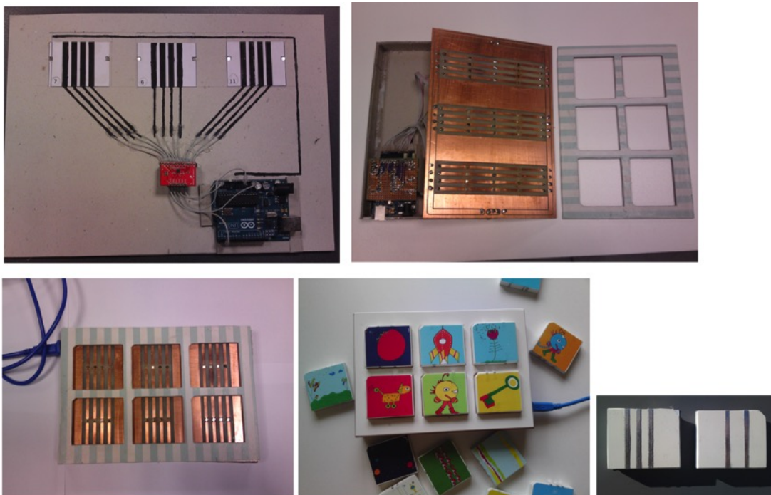
Figure 1-3 - Proof of concept (top left); first functional electronic prototype (bottom left); prototype with blocks (bottom centre) and backside of two blocks (bottom right).
