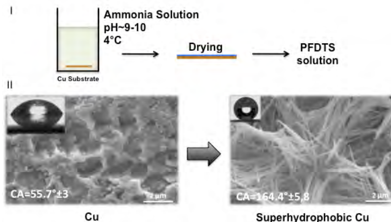
Figure 4.2. I. Schematic representation of the procedure to obtain Cu superhydrophobic surfaces. II. Cu substrate before film deposition, exhibiting CA around 56^\circ and after immersion in ammonia and PFDTs solution. On the surface of the Cu grew up micro and nano structures of \text{Cu}(\text{OH})_2 which combined with a PFDTs increased the water contact angle to ca. 164^\circ . Image adapted from [7].
