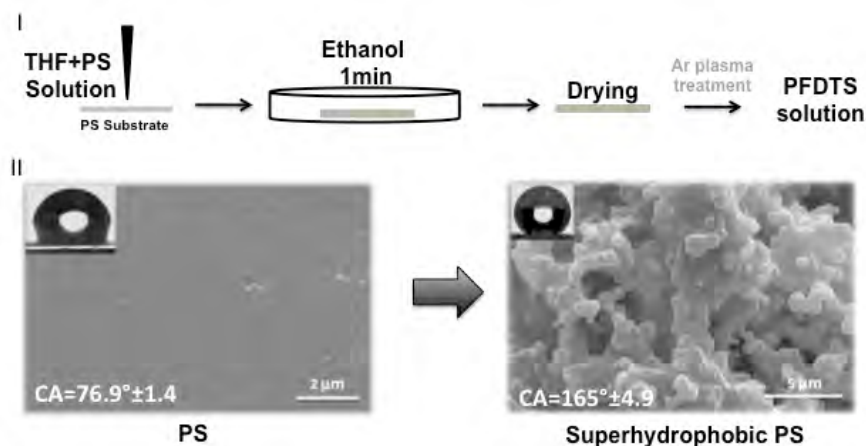
Figure 4.1. I. Schematic representation of the procedure to obtain PS superhydrophobic surfaces. II. Smooth PS exhibiting a contact angle (CA) of ca. 77^\circ (before modification) and the topographical structures of the superhydrophobic PS surface (after modification). The water CA achieved was higher than 150^\circ and the surfaces exhibited aggregates of nanostructures onto microstructures recreating the hierarchical structure of the natural water repellent systems. Images adapted from [7].
