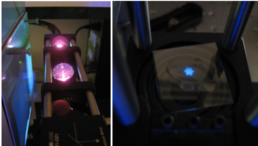
Figure 5.4 – Microstereolithography apparatus in operation curing a photo-sensitive resin
