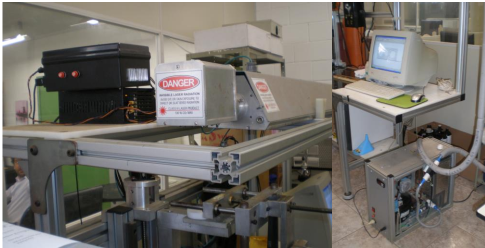
Figure 5.7 – CO 2 laser device: (a) gas tube and galvanometric mirrors; (b) power unit, control unit and water chiller
