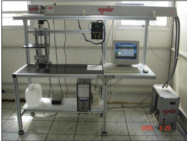
Figure 2.19 – Stereolithography system using infrared radiation [57]
