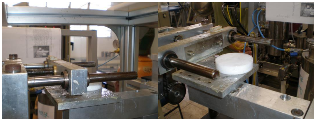
Figure 5.12 – Resin leveller; construction area
