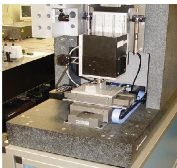
Figure 2.39 – Two photon polymerisation microstereolithography equipment developed at Laser Zentrum Hannover [92]
