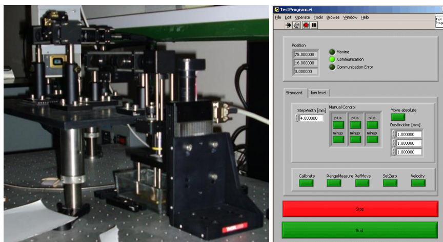
Figure 5.2 – Construction platform and MoCo control software
