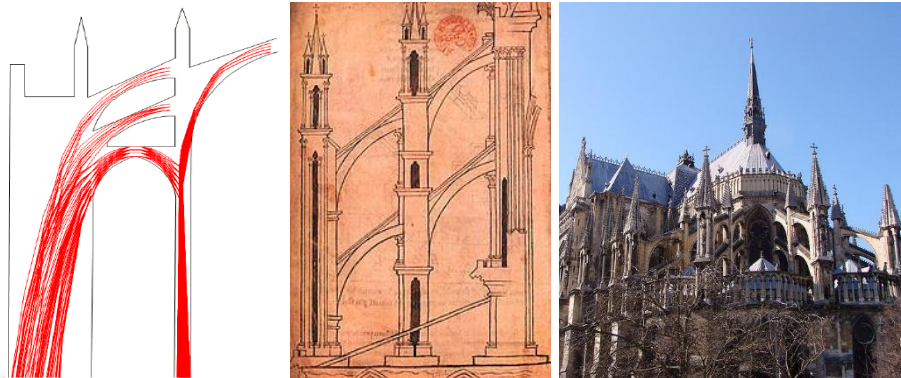
Figure 2-6. (Left) In the appearing typical section of a Gothic Cathedral, the upper flying buttress receives the lateral thrust from the weight of the roof, the wind and the weight of the clerestory wall, whereas the lower one counteracts the lateral outward forces from the weight of the nave vaults. Many possible thrust lines are shown (Luca et al. 2014). (Middle) Villard de Honnecourt's drawing of the flying buttresses system at Reims Cathedral ("Reims Cathedral" 2014). (Right) Exterior view of the east front of Reims Cathedral at Reims, France (1211-1275). System of flying buttresses ("Reims Cathedral" 2014).
