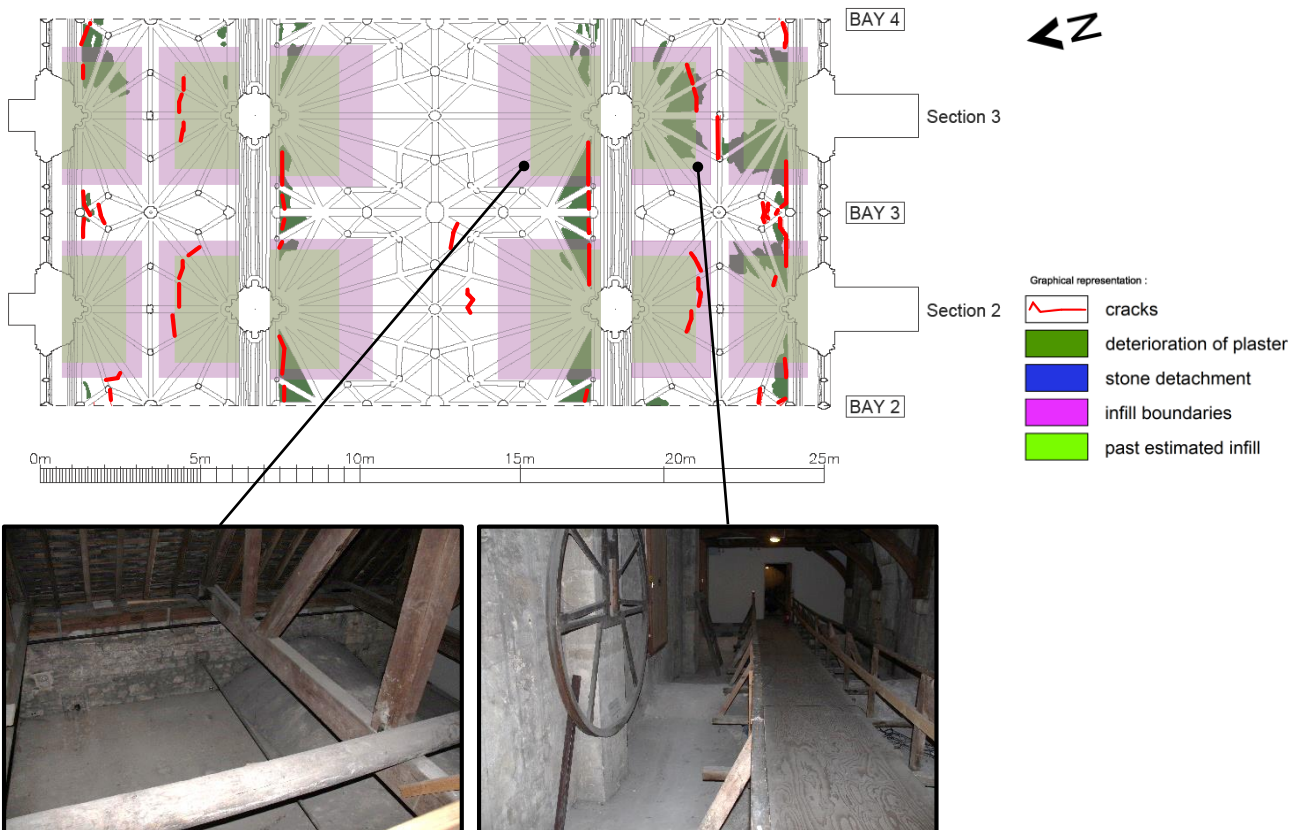
Figure 4-5. Damage map of the case study area, which depicts the current and former estimated infill boundaries.
