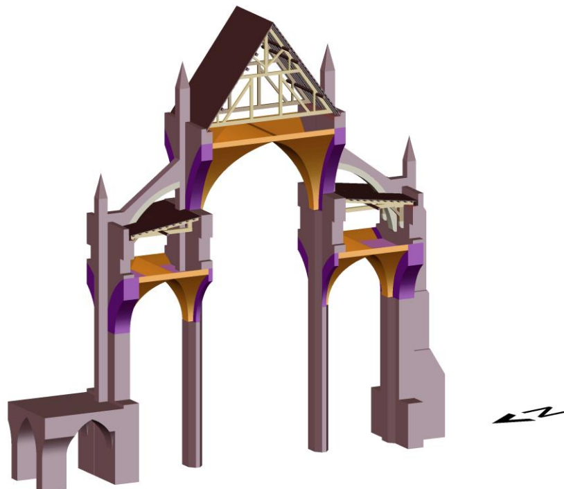
Figure 3-4. Generated geometrical model of the critical transverse cross section of Canterbury Cathedral's nave and the adjoining part of the cloister.
