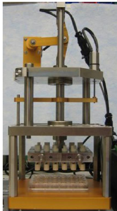
Figure 1.7- Example of bioreactor device for unconfined compression. Image taken from G.D. Nicodemus and S.J. Bryant [125], with permission of the authors.
