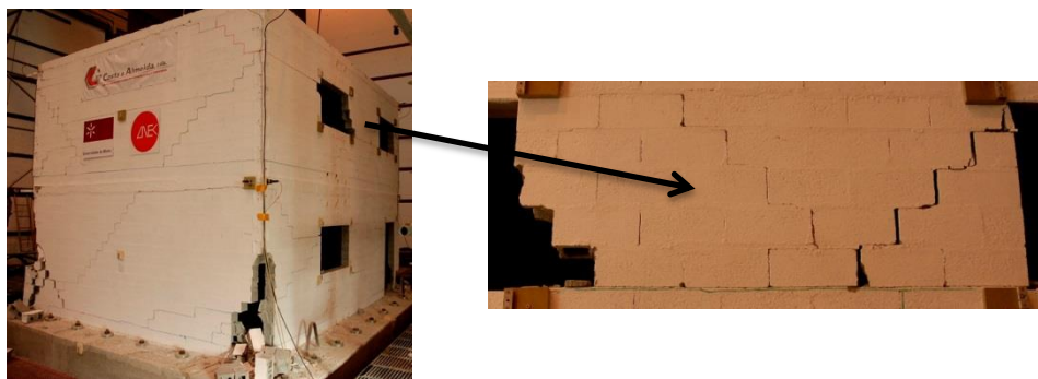
Figure 3.15 – Final damage west wall at second floor (between openings)
