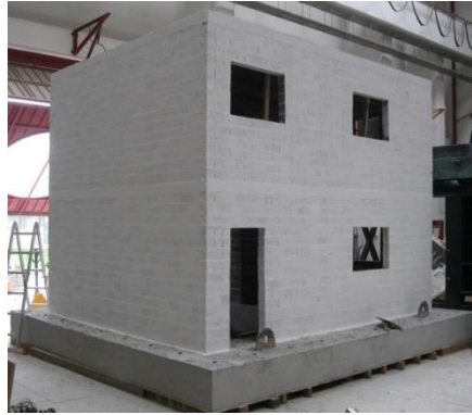
Figure 2.16 – Concrete block masonry building for experimental shaking table test
