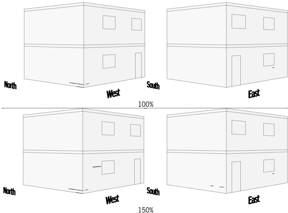
Figure 3.5 - Damage observed after each seismic input test for the RM model (100% and 150%)
