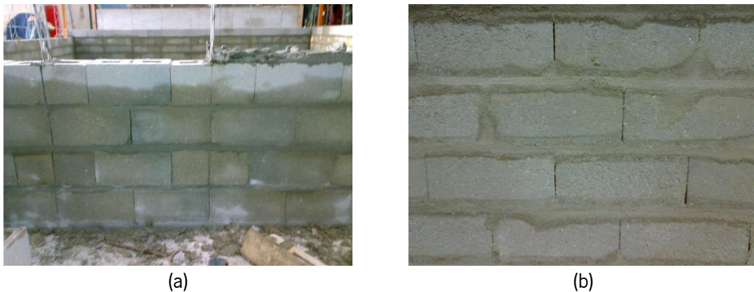
Figure 2.8 – Masonry bond patterns: (a) RM models and (b) UM models
