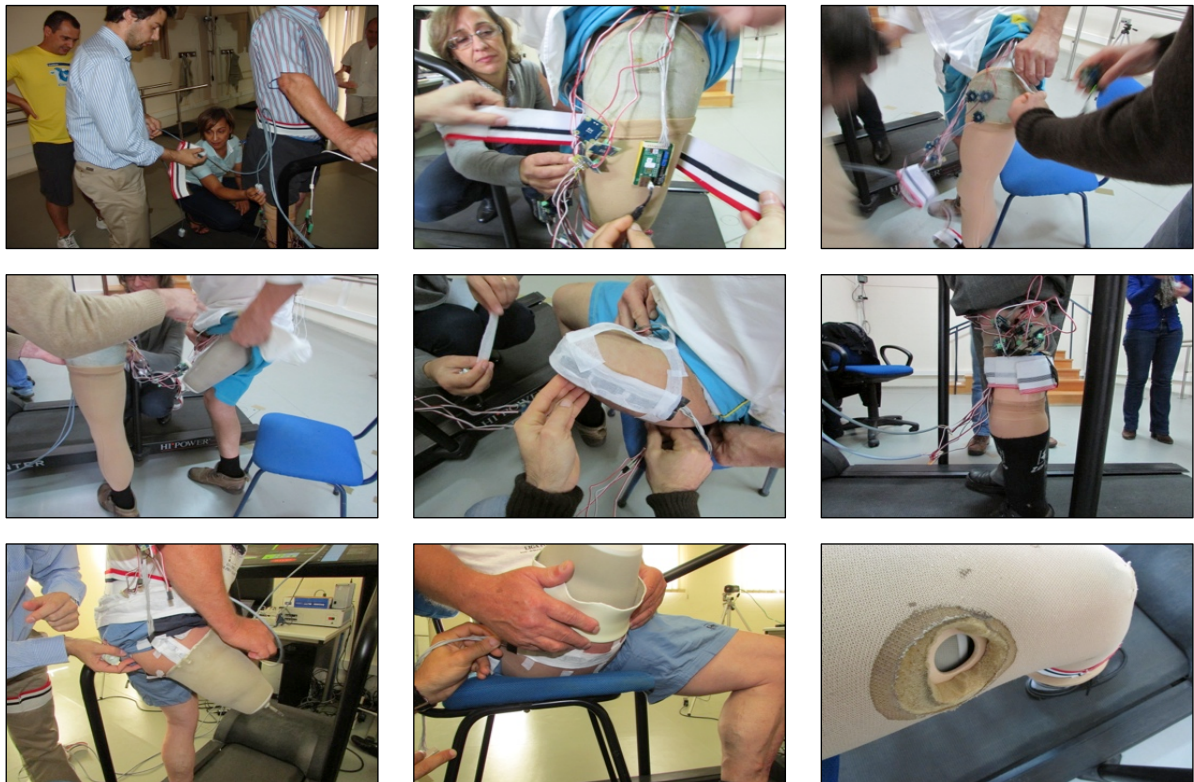
Figure 7.7: Pressure sensor prototype placement at the stump/sock/socket interface.
