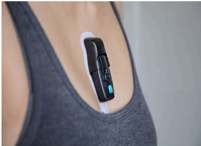
Figure 2 14-day ambulatory heart monitor (Preventice BodyGuardian Mini).
