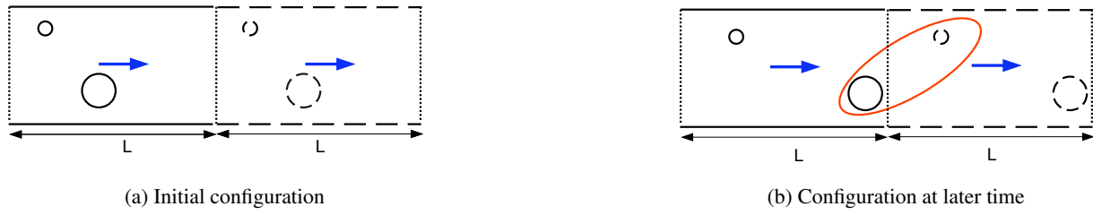
FIG. 3: Schematic of the formation of a periodic pair. Solid lines represent the actual simulation domain and particles; dashed lines represent the adjacent downstream periodic unit cell. Dotted lines indicate the periodic boundaries. The flow is from left to right. (a) Initial configuration of two particles in the staggered arrangement. (b) Pair formation between one actual particle and the periodic image of the other particle at a later time.
