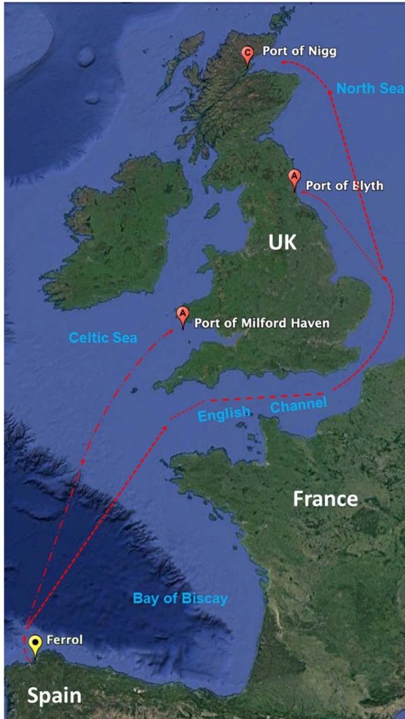
Fig. 12 Vessel transit routes from the floating platform fabrication yard to the offshore wind turbine assembly port (for illustrative purpose only)
