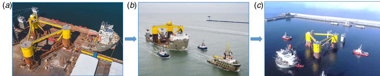
Fig. 3 Load-out and transport of floating platforms: (a) manufacturing port, platform load-out, (b) transporting platform by semi-sub HTV, tow to wind turbine staging port (Image source: Ref. [13]), and (c) float-off operation, the platform unit is released into the water at the staging port
