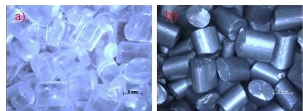
Figure 2 – a) Polystyrene b) PS coated with stainless steel film.
