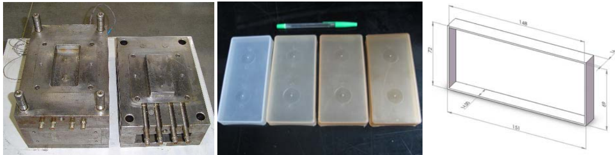
Figure 1. Hot runner mold, PP/nanoclay moldings and scheme of moldings with their dimensions.
