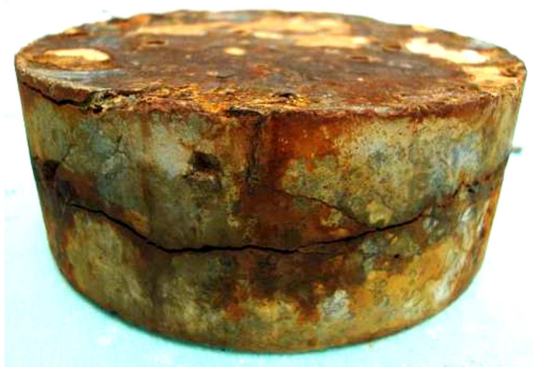
613 Figure B.15 - Micro-cracking observed in SFRSCC specimens after chloride migration test (a) and 614 fracture surface after diametral compression test (b)
