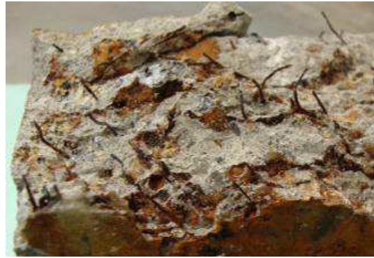
613 Figure B.15 - Micro-cracking observed in SFRSCC specimens after chloride migration test (a) and 614 fracture surface after diametral compression test (b)
