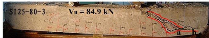
Figure 9 Comparison of crack pattern and failure mode of IS beams and SS beams: a) SS beams with 25 kg/m 3 steel fibres and b) IS beams with 25 kg/m 3 steel fibres
