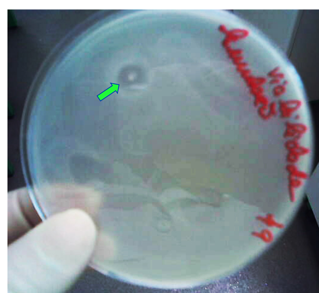
Figure 4. Petri dish after performance of the "spot" test to the nanoemulsion encasing bacteriophage T4.
