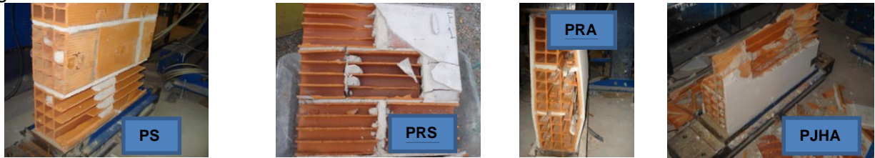
Figure 6. Specimens failure modes for compressive strength test
