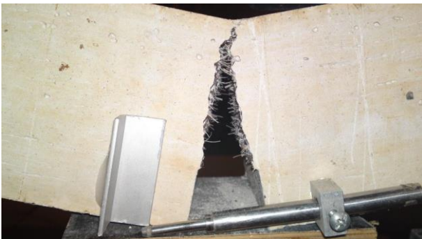
Figure 9. View of the crack after the fracture test in beam with composite material with sisal fibers
