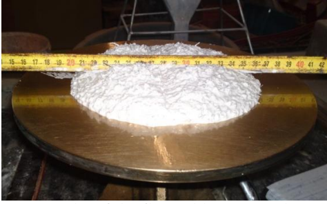
Figure 3. Results of the flow table tests to characterize the workability of the composite materials
