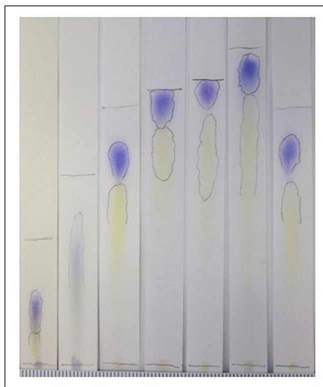
Figure 4. First six commercial papers (counting from left) with "questioned" sample (far right) using butanol as mobile phase and 90 minute elution. Pencil outline added to aid localization of spot.
