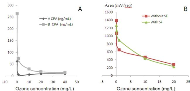
**Figure 1** - CPA degradation curves by ozone under two CPA concentrations (A) and with and without SF (B).
