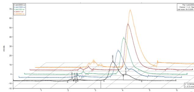
**Figure 2** – Chromatogram showing CPA degradation at 0, 1, 0.1, 10 and 20 mg/L of ozone.
