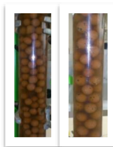
Figure 1. Picture of the columns with immobilised PP in LECA particles with different sizes.
