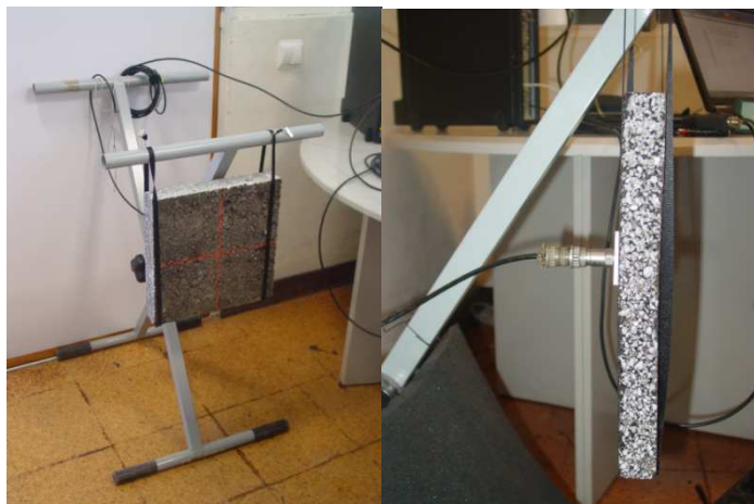
Figure 2 – Damping ratio testing set up
