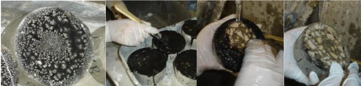
Figure 4 - Removal process of spray paint from the concrete surface protected with AGS 1
