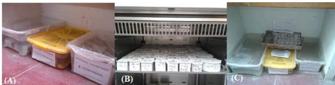
Figure 1: (A) Immersion in NaCl (B) Drying in carbonation chamber (C) Drying in laboratory environment
