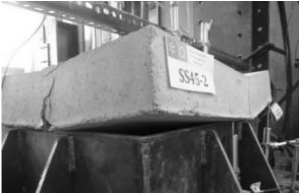
Fig. 12: Upward deflection of slab with respect to support line.
