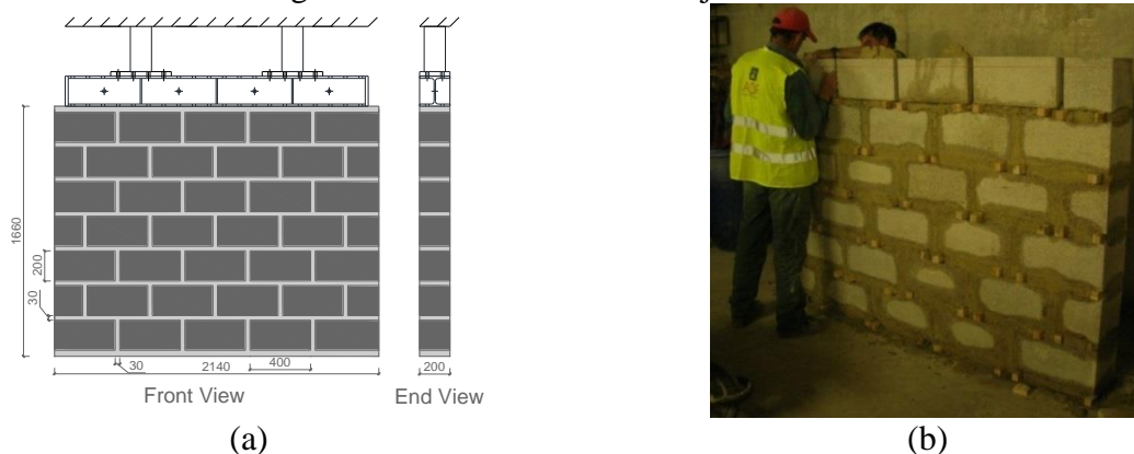
Figure 2 Regular masonry wall: (a) design, dimensions [mm]; and (b) construction in the laboratory
