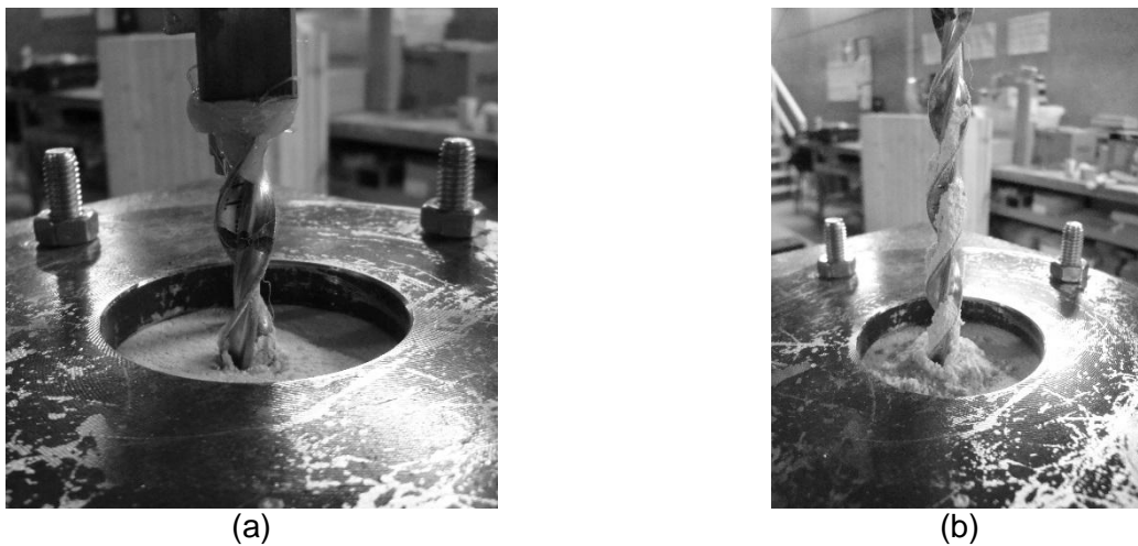
Figure 4. Pull-out failure: (a) beginning of test; (b) end of test.
