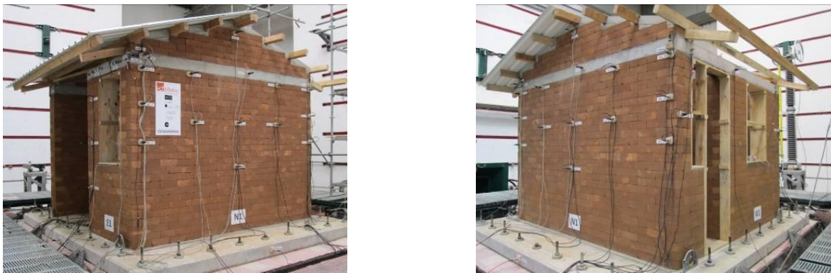
Figure 1. Earthen mock-up on the shaking table: North-East (left) and North-West (right) views
