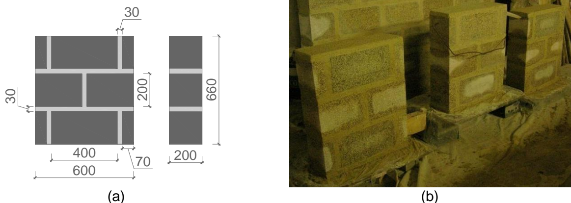
Figure 2. Masonry wallet: (a) design showing front and side profiles; and (b) completed construction of the three specimens [dimensions in mm]
