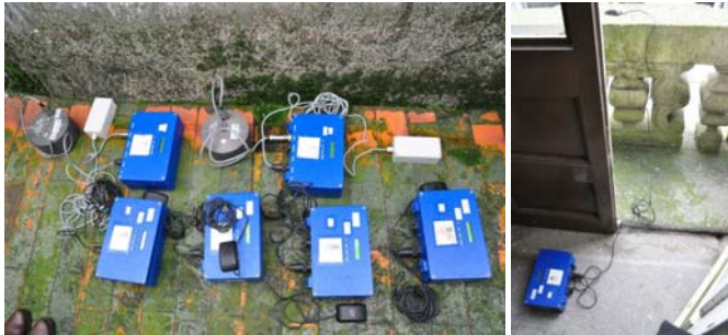
Figure 6. Six strong motion recorders.
