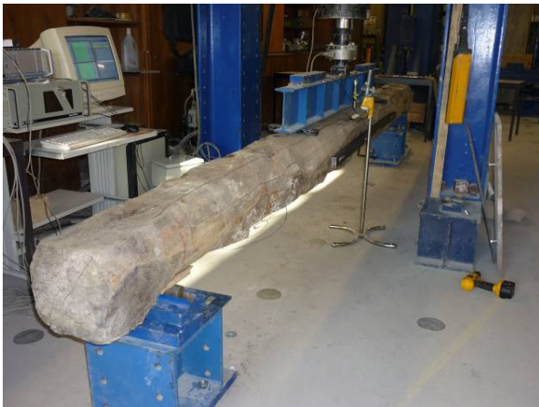
Figure 6: Beam B1 under a 4-point bending test
