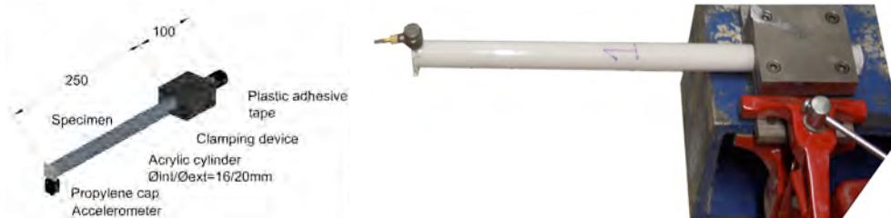
Fig. 1 – Experimental setup for EMM-ARM testing of epoxy adhesive [dimensions: mm]
