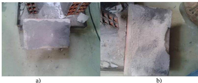
Figure 9: Specimens of hydraulic lime based mortars at 600°C: a) mortar with incorporation of 40% of PCM; b) mortar with incorporation of 40% of PCM and 1% of polyamide fibers.
