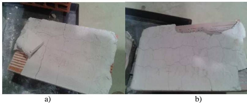
Figure 9: Specimens of gypsum based mortars at 600°C: a) mortar with incorporation of 40% of PCM; b) mortar with incorporation of 40% of PCM and 1% of polyamide fibers.
