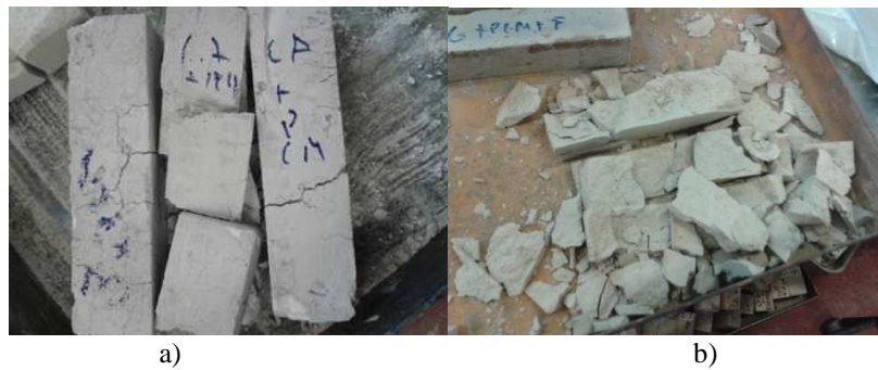
Figure 2: Specimens of aerial lime based mortars at 600°C: a) mortar with incorporation of 40% of PCM; b) mortar with incorporation of 40% of PCM and 1% of polyamide fibers.
