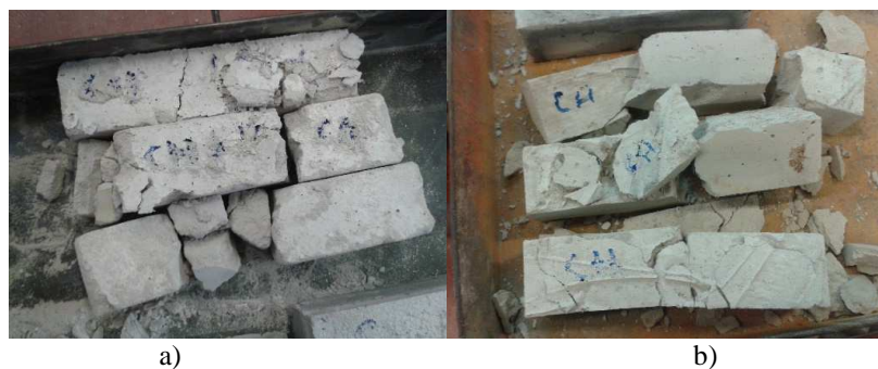
Figure 3: Specimens of hydraulic lime based mortars at 600°C: a) mortar with incorporation of 40% of PCM; b) mortar with incorporation of 40% of PCM and 1% of polyamide fibers.
