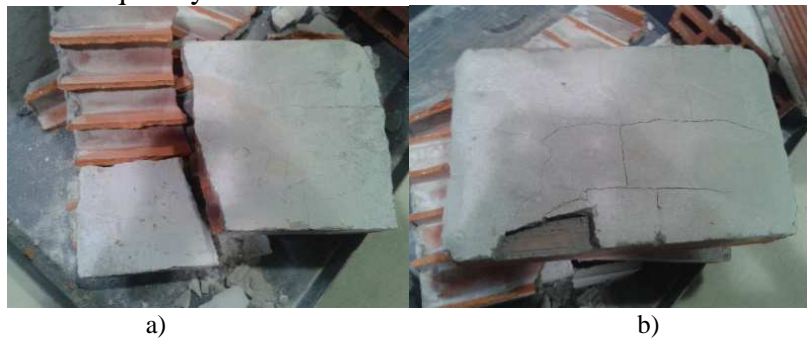
Figure 8: Specimens of cement based mortars at 600°C: a) mortar with incorporation of 40% of PCM; b) mortar with incorporation of 40% of PCM and 1% of polyamide fibers.
