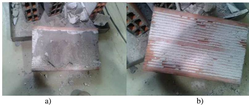
Figure 9: Specimens of aerial lime based mortars at 600°C: a) mortar with incorporation of 40% of PCM; b) mortar with incorporation of 40% of PCM and 1% of polyamide fibers.
