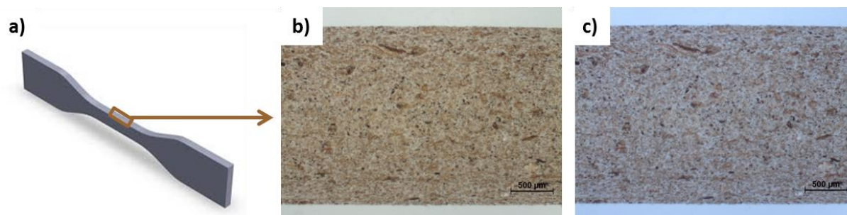
Figure 2.16. Optical microscopy of a cross-section of a polypropylene/cork (70/30) wt.%: (a) scheme of the tensile specimen revealing the longitudinal section; (b) image observed from the microscope in bright field and (c) image with color treatment to evidence the distribution of cork particles in the polypropylene matrix.
