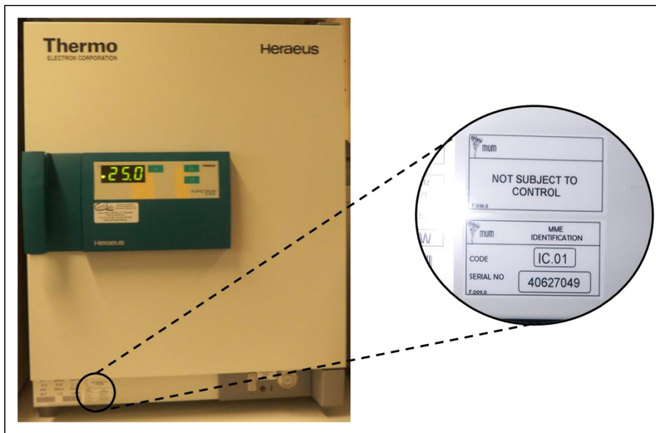
Figure 9 - Example of a label (F.038) used on an incubator (IC.01) from Micoteca da Universidade do Minho not subjected to control or calibration, placed together with F.009.
