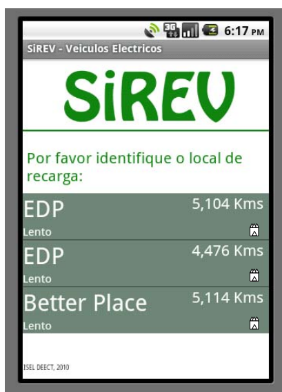
Figure 6-24: Recommendation, because SiREV detects that range is below the configured limit of 30 km
