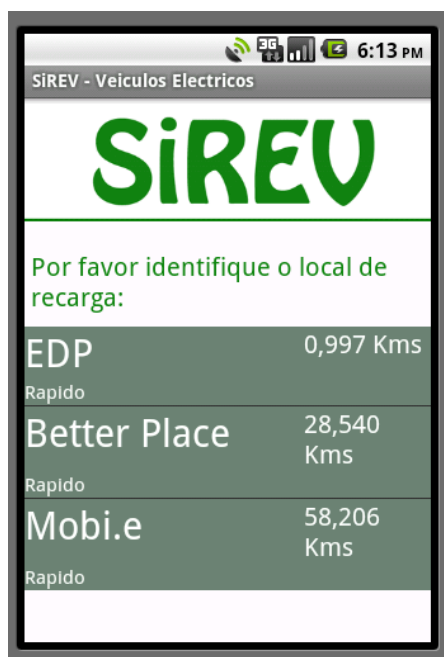
Figure 6-23: Recommendation generated because SiREV detects that EV range is below 30% of initial range
