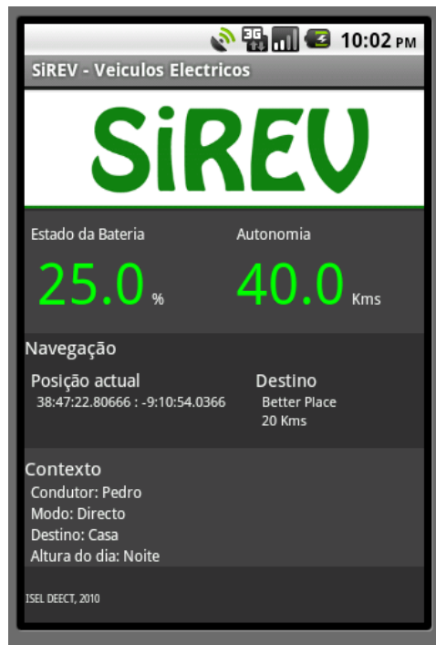
Figure 6-17: SiREV: Charging indication (SOC); EV estimated autonomy; A charging place identified (Better Place) at 20 km; and the Context Information (driver, mode, destination and day period) (in Portuguese language)
