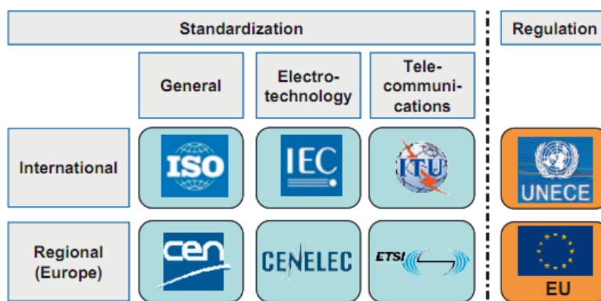
Figure 2-21: Main components of the standardization landscape and their interrelationships together with their regulatory body
