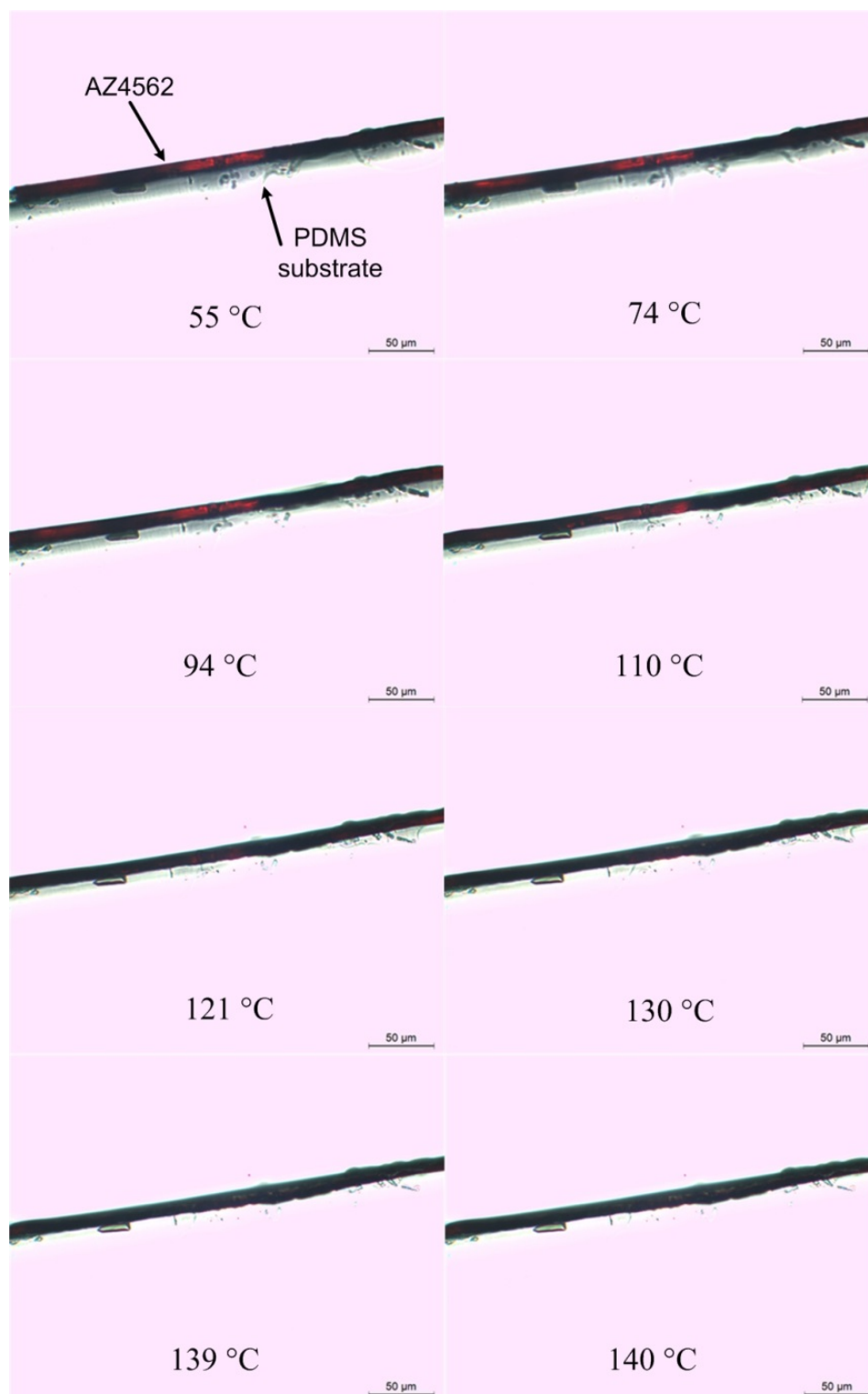
Figure 4.26 – Snapshots of the AZ4562–PDMS interface taken with the sample being heated-up at a temperature profile similar to the one used during the thermal reflow. The scale in the pictures represents 50 \mu\text{m} .
