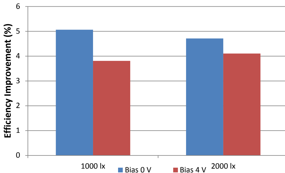
Figure 4.46 – Efficiency improvement (%) achieved at different illuminance values (red light) and reverse bias voltages by the developed MLs fabrication process on a 240 \mu\text{m} square PD.
