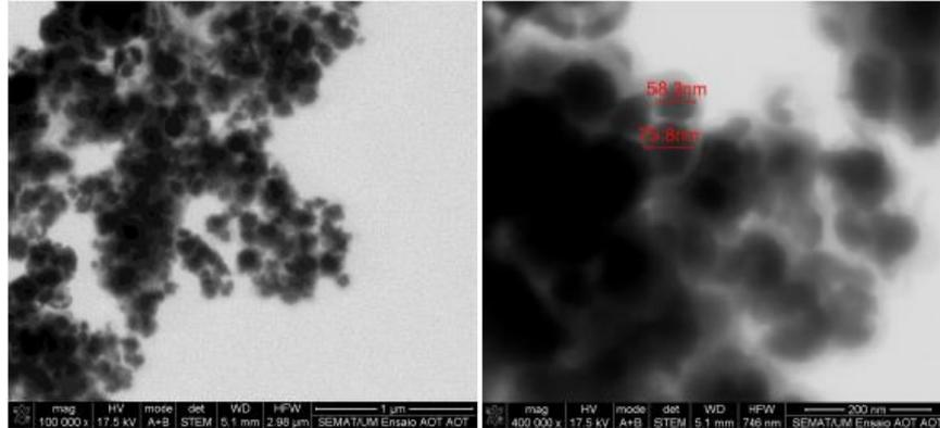
**Figure 1.** SEM images of dry magnetoliposomes of nickel nanoparticles covered by the double chain surfactant AOT (sodium bis(2-ethylhexyl) sulfosuccinate).
