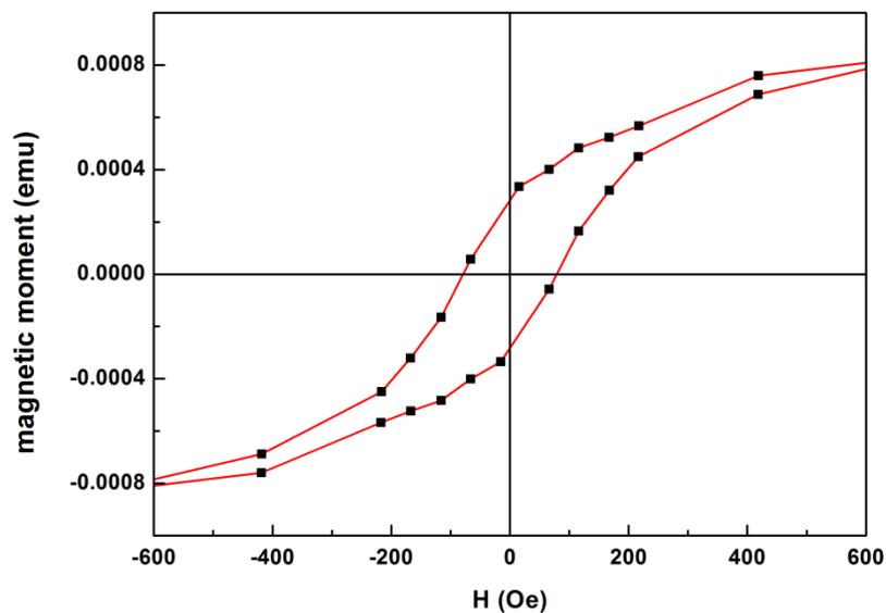
**Figure 2.** Hysteresis loop of Ni nanoparticles at room temperature obtained by SQUID.
