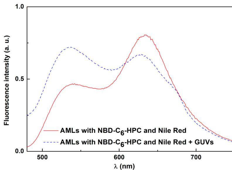
**Figure 3.** Fluorescence spectra ( $\lambda_{exc}=400$  nm) of AMLs of egg-phosphatidylcholine with Ni/silica core/shell nanoparticles with Nile Red ( $2 \times 10^{-6}$  M) and NBD- $C_6$ -HPC ( $10^{-6}$  M); and with GUVs.
